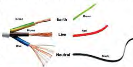
Fig 8.22 Three types of coloured wire
