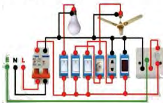
Fig 8.24 Connection of the bulbs in household electrification
